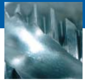
■ Cutting edge after 1,000 holes tapping
